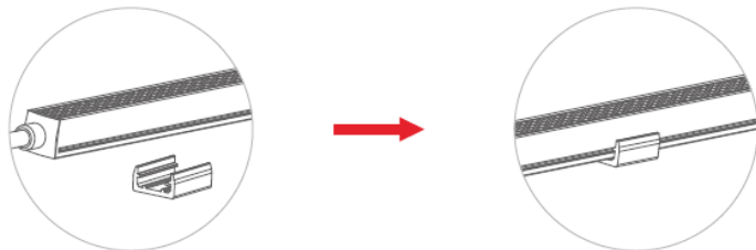
Fixed by aluminum profile and screw
